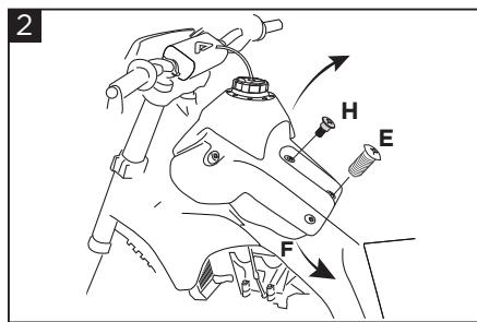
**Remove screws (H) and (E) from the tank and disassemble it from the motorcycle. Remove the original pump (F).**
