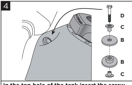
**In the top hole of the tank insert the screw (D), the bushings (C) and the rubbers (B) as shown in the figure.**
