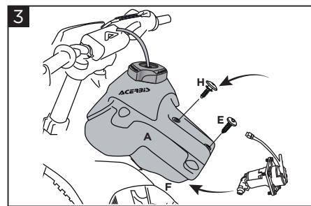
**Mount the pump (F) on the Acerbis tank. Position the Acerbis tank (A) and fasten the screws (H) and (E).**
