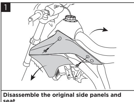
**Disassemble the original side panels and seat.**
